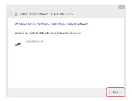
At the procedure ending, click on **Close**, then disconnect and reconnect the FDM-S2 on the same USB port. Now the USB driver of the FDM-S2 is installed on your computer.
