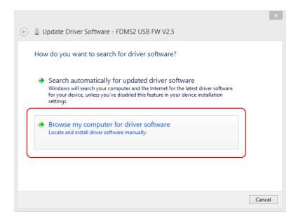
In the next window, insert the driver folder location using the **Browse** button and check the option **Include subfolders**, in this way the manual driver search is enabled. Select the folder: **C:\Program Files** (x86)\ **ELAD\FDM-SW2\ELAD\_FDM\_Driver** then click **Next**.
